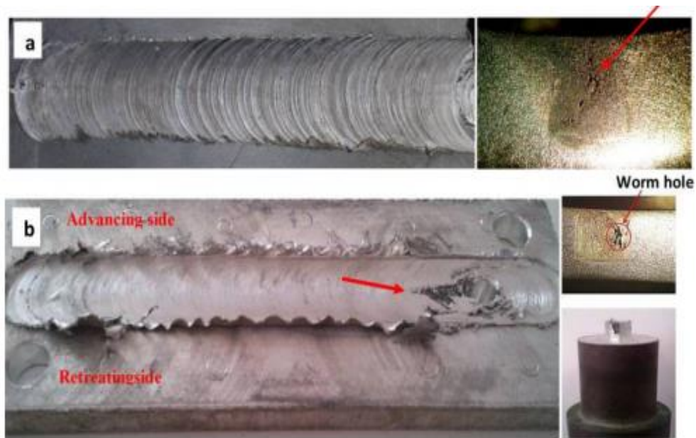
Figure:9 Samples of friction stir welding with 800 rev min 21 and 1600 rev min 21 and 40 mm min 21 translational speeds(Rouhi, Mostafapour and Ashjari, 2016).
