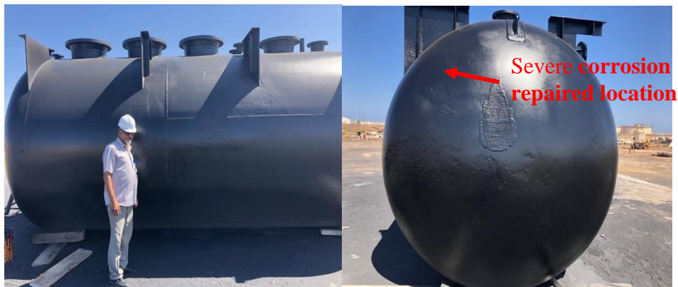
Figure 4: Tank condition after completion of all necessary maintenance activities
