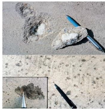
Figure 2: Physical popout (top); ASR popout (bottom) [2].
