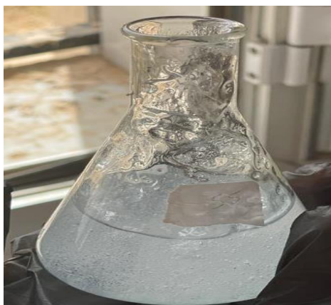
Figure 4: 2% of the prepared Carbopol 940 polymer gel.
