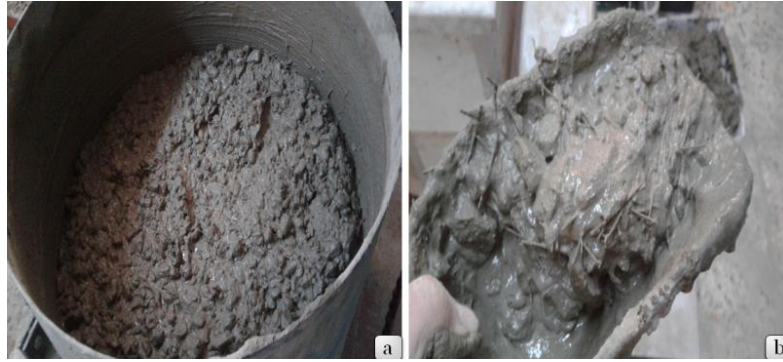
Figure 3: Homogenous fresh steel fiber reinforced concrete after mixing
