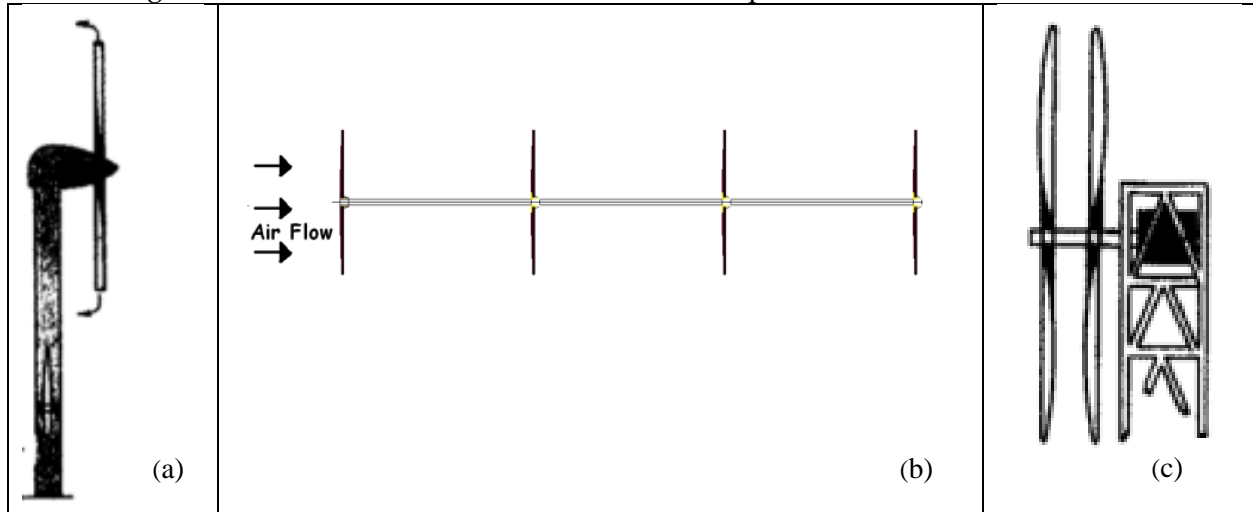
Figure 2: The previous technology as (a) The Enfield-Andreau type of Horizontal Axis Wind Turbine (HAWT), (b) the multiple rotors in the same plane on a single tower and (c) wind turbine composed of counter-rotating blades.
